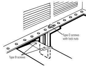
Adjust the carriage bolts and the lock nuts in each support so that the case is installed with a slight downward tilt (about 1/4") toward the outside. Tighten the bolts.
